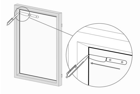
Mark the distance the blade travels under the gasket.
