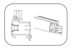
**3.** Apply pressure to ensure strip adheres to ledge. Brush strip should protrude from top edge of headrail.
