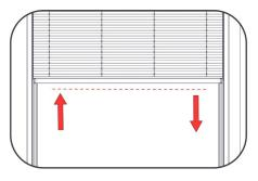
**11.** To align the bottom rail horizontally, simply pull it into the position desired. It will stay in position under tension from the cords.
