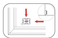
**4.** Position bracket behind the rubber bead and push until the metal leg is behind the bead. Check bracket is parallel to bead and is securely fitted. Repeat for the other side.
