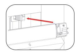
**9.** Align headrail endcaps with top corner fixing brackets and push fully home.
