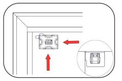
**2.** Position bracket behind the rubber bead and carefully push until the metal legs are behind the rubber bead. Check bracket is square to the sides of the bead and it is secure. Repeat for other side.
