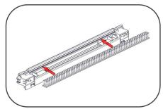
**2.** Insert brush strip to upper ledge on inside of headrail.
