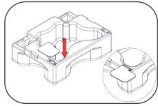
**3.** Place the bottom corner bracket into the slot on the fitting tool.
