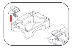
**1**. Place the top corner bracket into the slot on the fitting tool.
